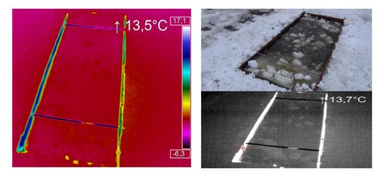
Apparently no oil detected in basin B but temperature difference between water and ice was observed
